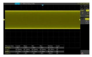
At any one timebase, ADS-4000 can measure using all 14M sample points. This ensures the accuracy of measurements while the math coprocessor decreases measurement time and increases ease-of-use.
