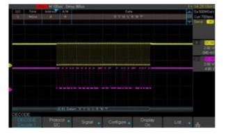
Serial bus decoding function (Standard)
