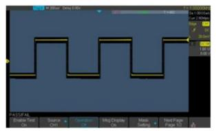
The ADS-4000 utilizes a hardware-based Pass/Fail function, performing up to 40,000 Pass / Fail decisions each second. Easily generate user-defined test templates provide trace mask comparison making it suitable for long-term signal monitoring or automated production line testing.
