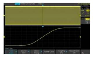
Using hardware-based Zoom technologies and a record length of up to 14 Mpts, users are able to use a higher sampling rate to capture more of the signal and then quickly zoom in to focus on the area of interest.
