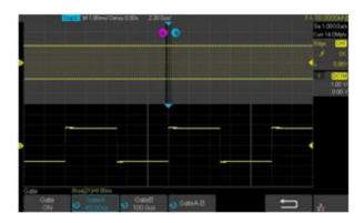
Through Gate and Zoom measurement, you can specify arbitrary waveform interval of data analysis and statistics to avoid measurement errors caused by invalid data.
